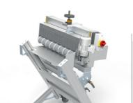
The brush placed over the spiral roller prevents the sprues from passing above the roller itself
