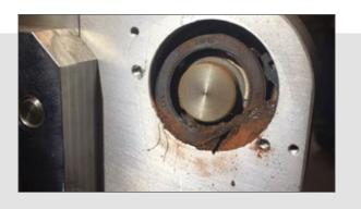
This photo shows a drive roller shaft damaged by electrostatic charges
