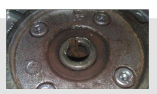
The photo highlights the harmful effects that electrostatic charges can have on the drive roller: the drive key housing is completely damaged
