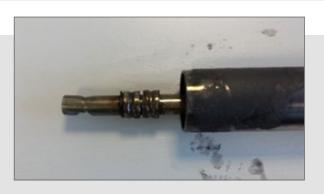
This photo highlights the harmful effects that electrostatic charges can have on the conveyor drive roller shaft
